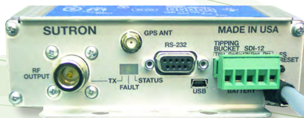
USB Mini Type B requires USB Type A Transition Cable. Sutron provides 6 ft USB Cable upon request. Cable Part # 6411-1613
